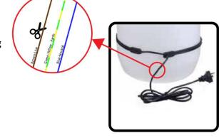
**Step 3.** Divert the active wire into the blade connects (terminals 4 and 5 shown below)
